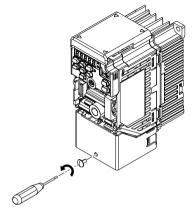
Figure 5.13 Remove the Screw that Attaches the Front Cover of the Conduit.
