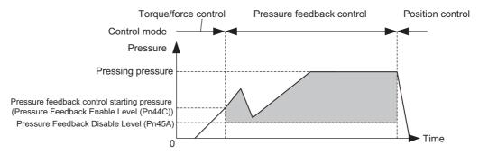
Note 1. Pressure feedback control is enabled in the gray area in the above figure.
