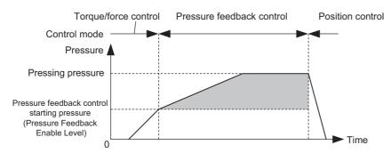
Note: Pressure feedback control is enabled in the gray area in the above figure.
